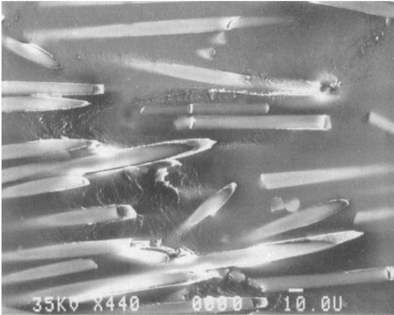
f. Interconnection of local & fiber-end cracks
